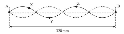
The positions of maximum and zero displacement for one overtone are shown. Points A and B are fixed. Points X, Y and Z are points on the string.
